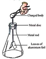
It consists of a metal rod. At one end of the rod, two leaves of aluminium foil are fixed and at the other end, there is a metal disc. The leaves of aluminium foil are placed inside a conical flask and the flask is corked to isolate the leaves from air.
